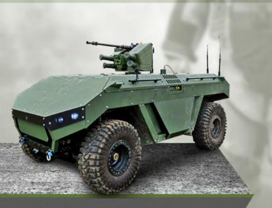
PIAP HUNTER reaches a maximum speed of up to 50 km/h. Equipped platform was equipped with six high-resolution cameras.
