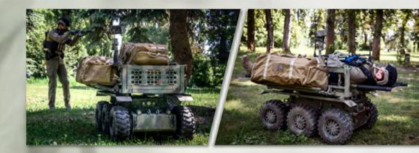
The PIAP IBIS robot can be controlled from the PIAP HUNTER robot control panel and can serve as observation support thanks to the installed PTZ head with a day-night camera with zoom and a thermal imaging camera. Radio control of a smaller robot in a network with a PIAP HUNTER combat robot allows for mutual transmission of a radio signal, extending the operational range of one or the other unmanned platform.
