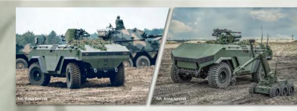
The vehicle is equipped with a 3-link dependent suspension with a Panhard rod coil springs and shock absorbers with controlled damping. Łukasiewicz-PIAP used a differential lock and two steering axles.
