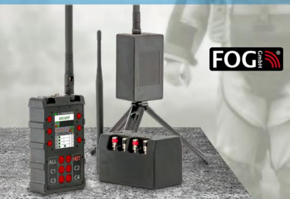
The transmitter is equipped with a high-resolution transflective display that allows you to read the most important information such as network conductivity, battery charge, range strength, and security status. Thanks to the variety of transmitters - single-channel, single-channel lightwaight, four-channel, ShockTube - you can plan activities to minimize the necessary amount of equipment and space.
