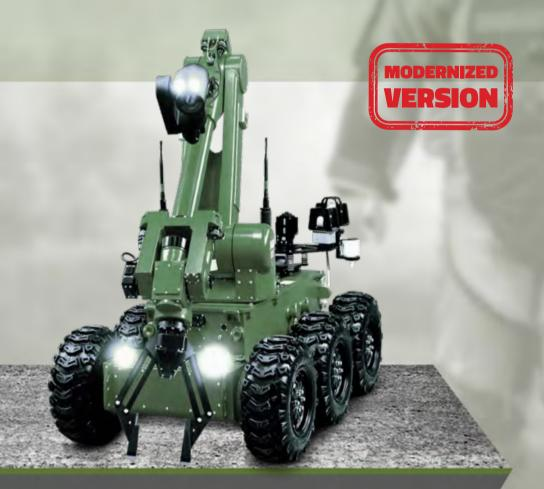
PIAP IBIS® is a fast robot (10 km/h). Special design of mobile base suspension ensures optimum wheel contact with the ground. Precision drive system ensures fluidity of the movement of every part of the robot, at any speed.
